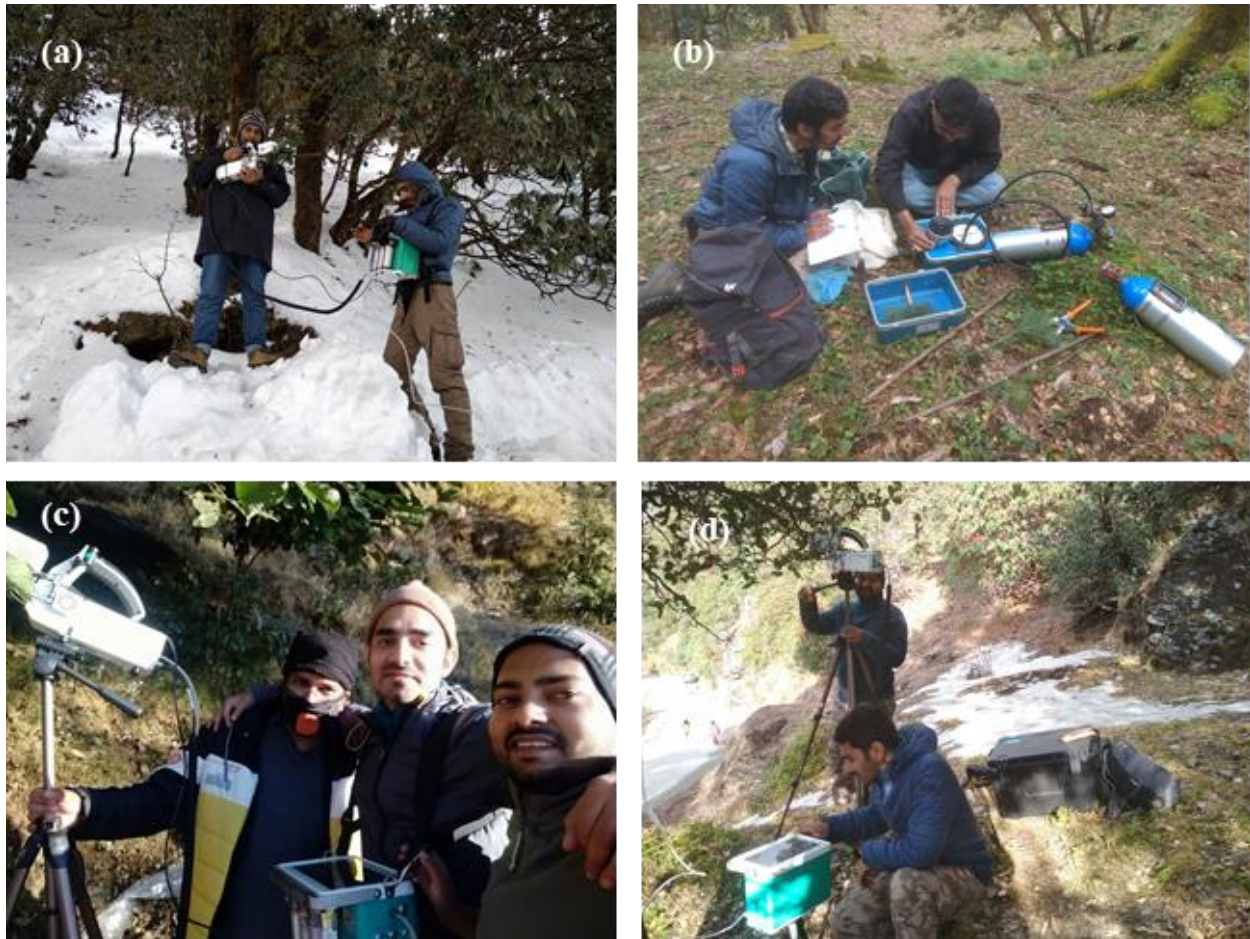
Figure 11 (a). Sampling with LiCor-6800, for leaf gas exchange measurements during winter. (b). Sampling with PMS 600 for plant water potential measurements. (c). After sampling time with the team. (d). During measurements of leaf gas exchange for spring season.
